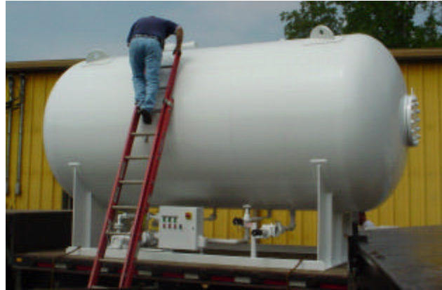
Refurbished 4,200 gallon R-134a storage system with special pump package.
